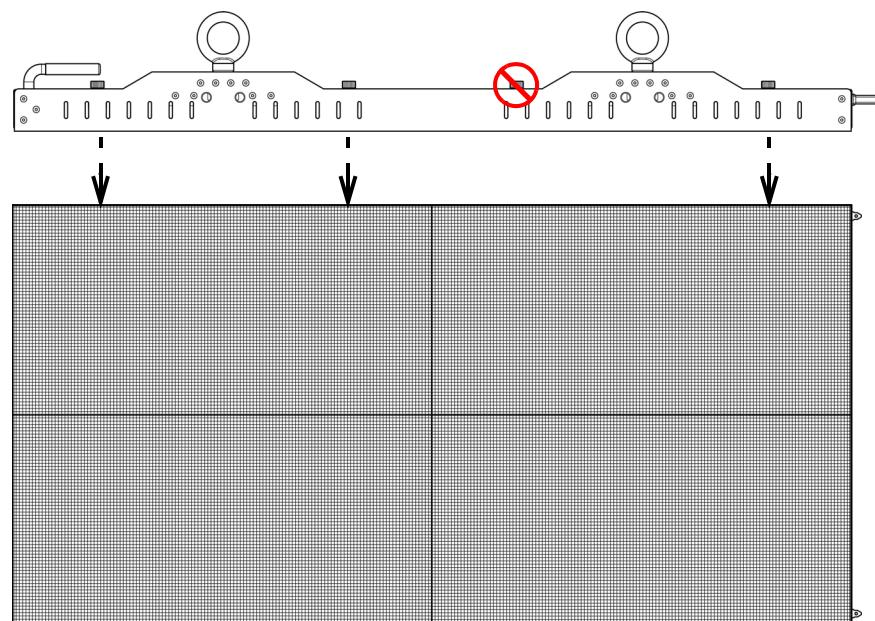
The F4 IP can be mounted horizontally with the RB-F100CM Rig Bar. Follow the same instructions as in [Rig Bar/Panel Assembly](#), but take extra care, as the long side of the product has neither alignment conicals nor magnets. When mounting horizontally with the RB-F100CM, one of the Rig Bar Speegos will not be used.
