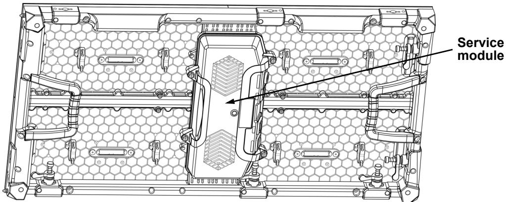
The F4 IP service module can be accessed and serviced from either the front or the rear of the panel at any time, so a technician does not have to walk around an entire video wall multiple times to service a single panel. Follow the instructions below to access the F4 IP service module from the front of the panel:
