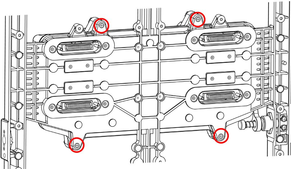
2. Remove the four screws from the rear of the panel by turning the screws clockwise from the front of the panel.
