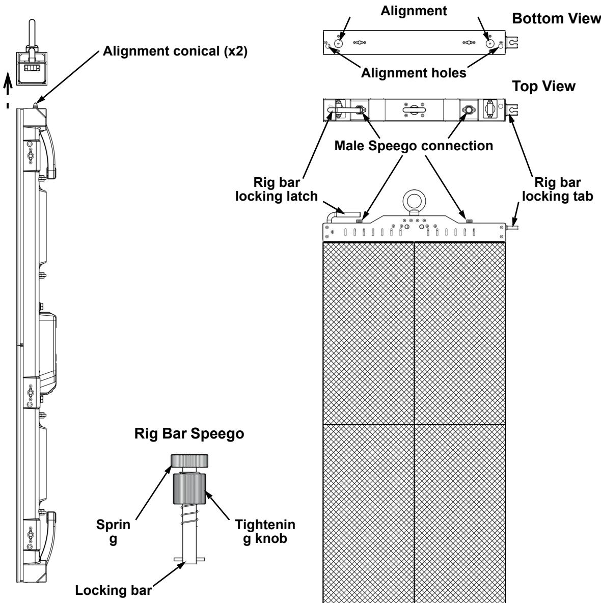
1. Insert alignment conicals into the alignment holes and allow magnets to connect.
