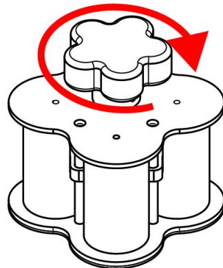
The MT-01 is specially designed to carefully remove and replace the F4 IP LED module from the front while the panel is mounted in a video wall setup. Before using this tool, be sure that the magnet is drawn all the way back to the home position by turning the knob clockwise. Failure to set the magnet to the home position may result in damage to the module.
