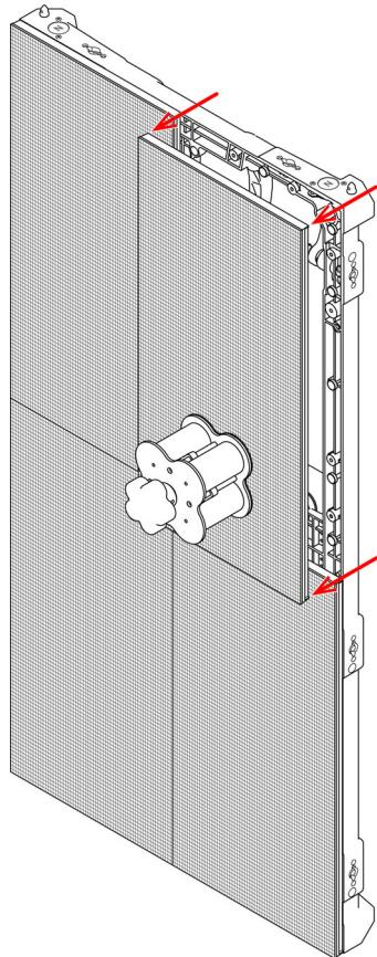
3. With steadily increasing force and keeping as straight as possible, pull the MT-01 back until the module is released from the frame.
