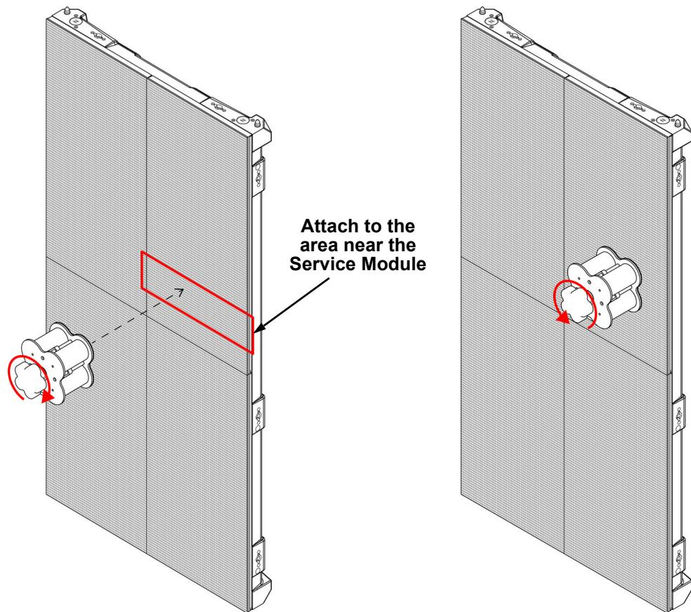
2. Carefully place the MT-01 against the module in the open position (with the knob turned clockwise), then turn the knob counter-clockwise until the magnet is 1 mm away from the module.
